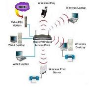
Fig. 1. Wireless Networking Design.
